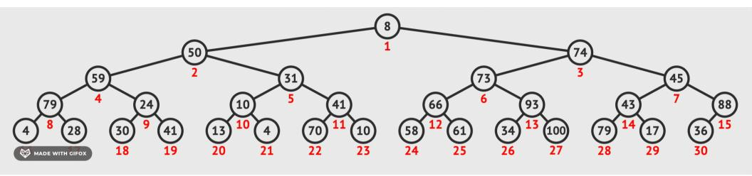
**High-level approach:** Given an arbitrary vector of keys. Starting from the internal node with the largest index in the vector, and moving upwards in the tree through all the internal nodes (level by level), sift the root of each subtree downward as in the **bubble-down process** until the **heap property** is restored.
