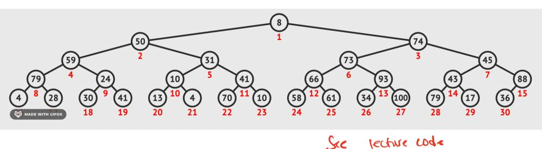
**High-level approach:** Given an arbitrary vector of keys. Starting from the internal node with the largest index in the vector, and moving upwards in the tree through all the internal nodes (level by level), sift the root of each subtree downward as in the **bubble-down process** until the **heap property** is restored.
