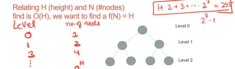
How many nodes are on level L in a completely filled binary search tree?
