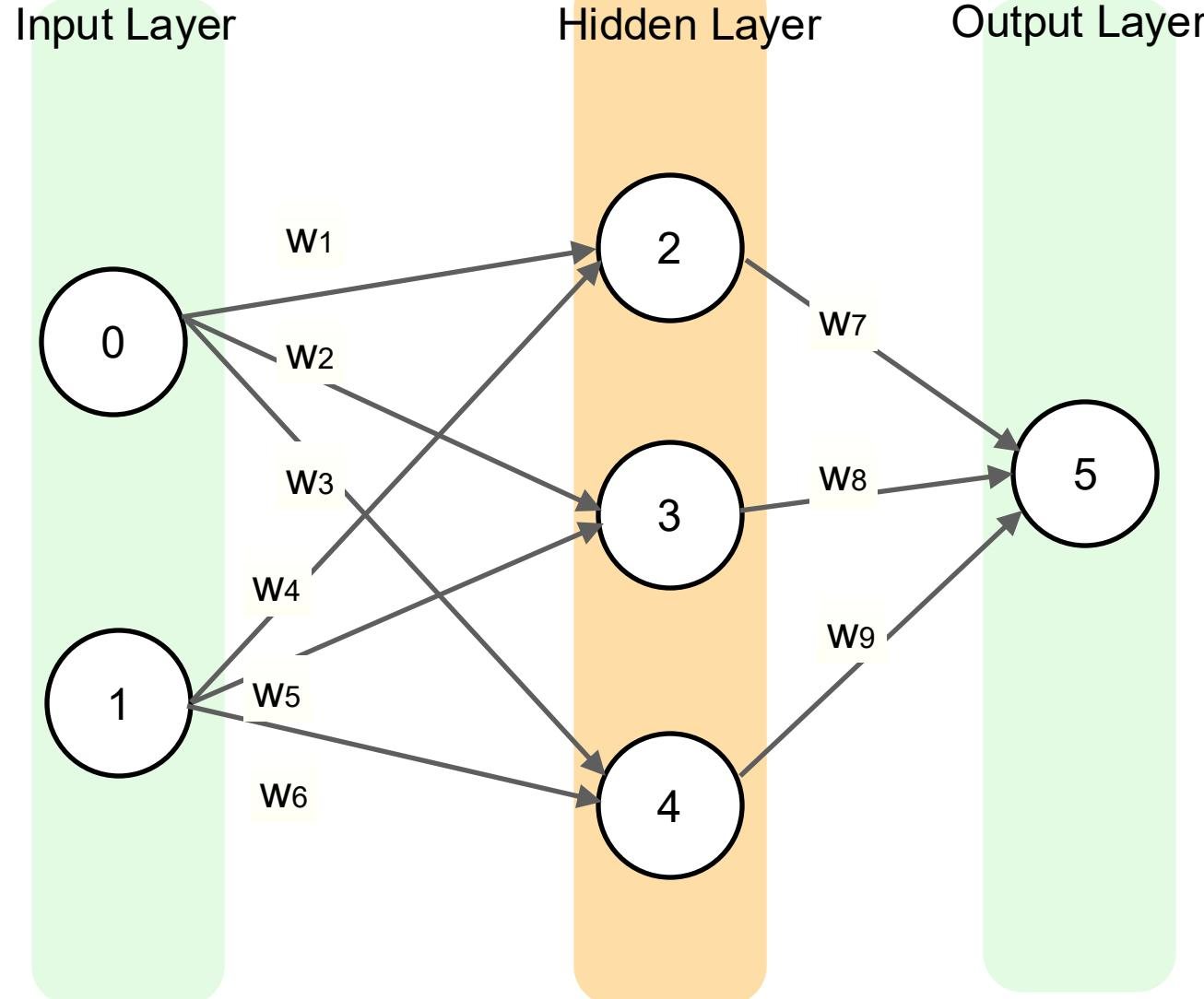
A **feedforward neural network (FNN)** is the simplest type of neural network where data flows in one direction — from input to output — without looping back.
