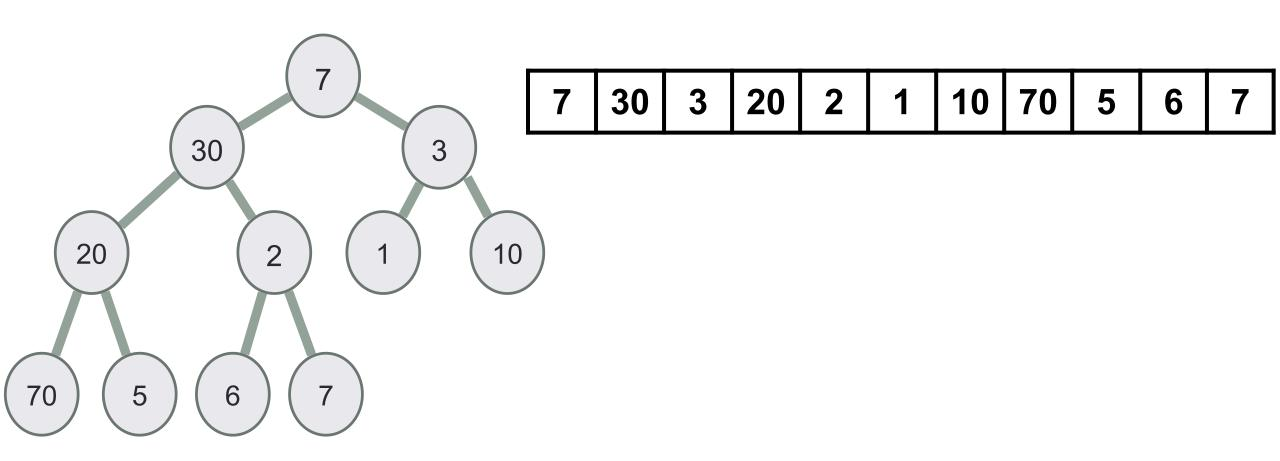
**High-level approach:** Starting from the level containing the last internal node and moving upwards through all the internal nodes, sift the root of each subtree downward as in the **bubble-down process** until the **heap property** is restored.
